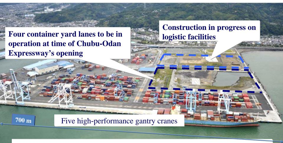
Two fifteen-meter-deep berths lined side-by-side Earthquake-resistant wharves, seven hundred meters in length
